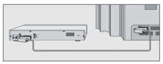
1 Connect the »AV1« or »AV2« television sockets and the corresponding sockets of the video recorder, DVD player or the SET-TOP box with a Euro-AV (Scart) cable.
